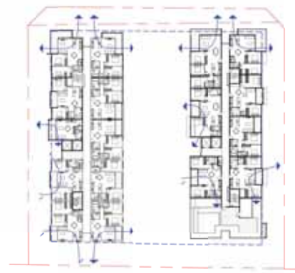
4 CROSS VENTILATION DIAGRAM - L4 1 : 500
